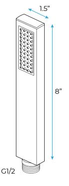
Flow Rate: 2.0 GPM / 7.6 LPM
